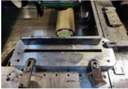
Wirecut Profile Machining for Copper Extrusion Die
