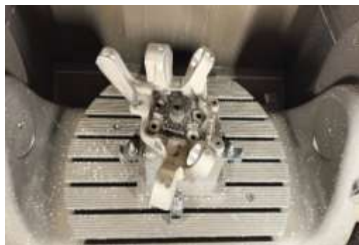
Steering Knuckles Machining for TATA ROWA Project on CNC 5 Axis Milling Machine
